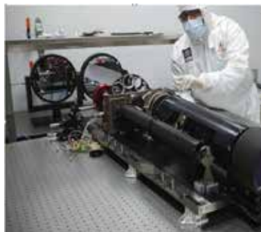
MCNS faculty working in a class 100 clean room at ISRO Bangalore: developing SUIT onboard Aditya-L1
