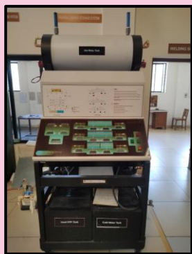
Thermal energy storage system
