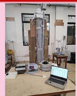
Thermosiphon heat transport device
